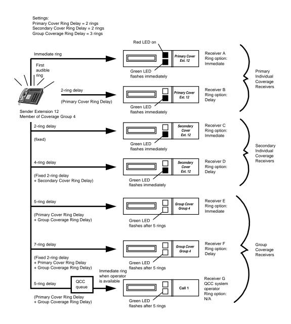
Figure 9. Individual (Primary and Secondary) and Group Coverage Ringing Patterns
