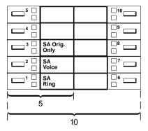
Figure G-7. MLX 5- and 10-Button Telephones (Hybrid/PBX Mode)
