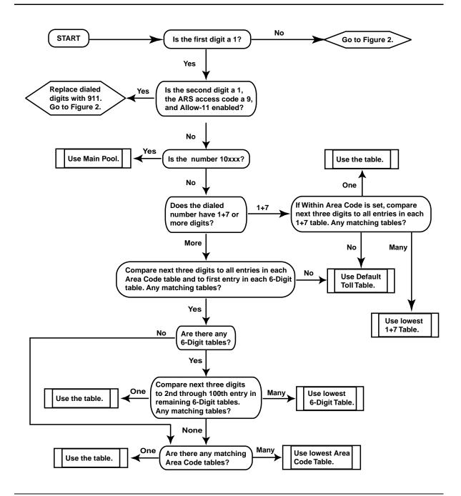
Figure 1. ARS Search Algorithm When Leading "1" is Dialed
