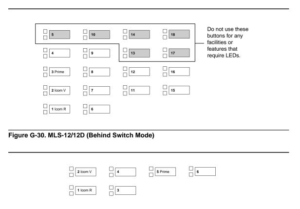
Figure G-31. MLS-6 Telephone (Behind Switch Mode)
