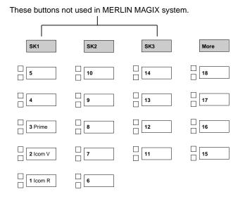
Figure G-26. ETR-18/18D Telephone (Behind Switch Mode)
