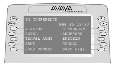
Figure 19. 7-Line 4424LD+ Telephone Display Home Screen (MERLIN Messaging 2.0 or Earlier)
