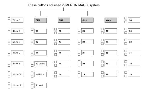
Figure G-18. ETR-34D Telephone (Key Mode)
