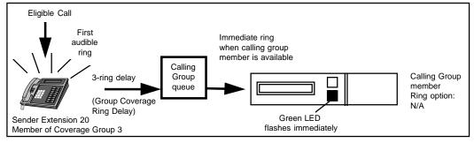
Figure 8. Group Coverage Only or All Individual Coverage Receivers Unavailable
