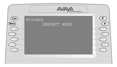
Figure 23. 7-Line 4424LD+ Display Inspect Screen for Programmed Button
