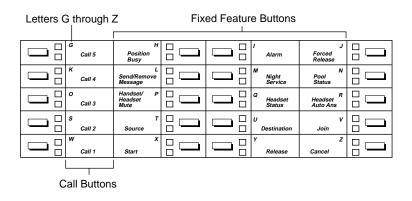
Figure 36. QCC Button Assignments for an MLX-20L Telephone
