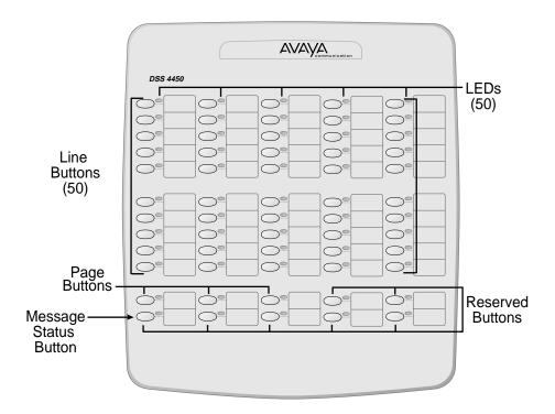
Figure 15. Direct Station Selector (DSS)
