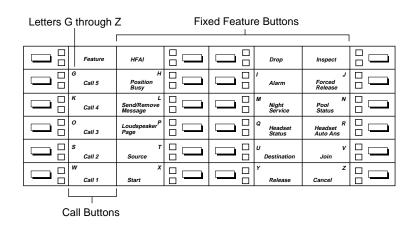
Figure 35. QCC Button Assignments for a 4424LD+ Telephone
