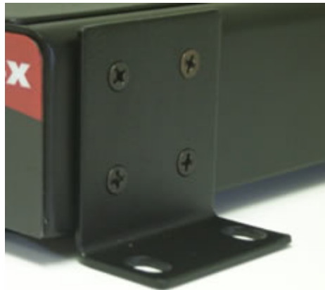
Figure 4: Wall Mount Bracket Installation
